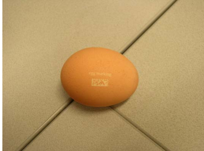
Figure 2.53: Egg marking, ablation [ 3 rd Nd:YAG laser, 355 nm].
