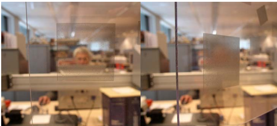
Figure 2.39: Louvre film in 3 mm thick polycarbonate [ Q -switched Nd:YAG laser].
