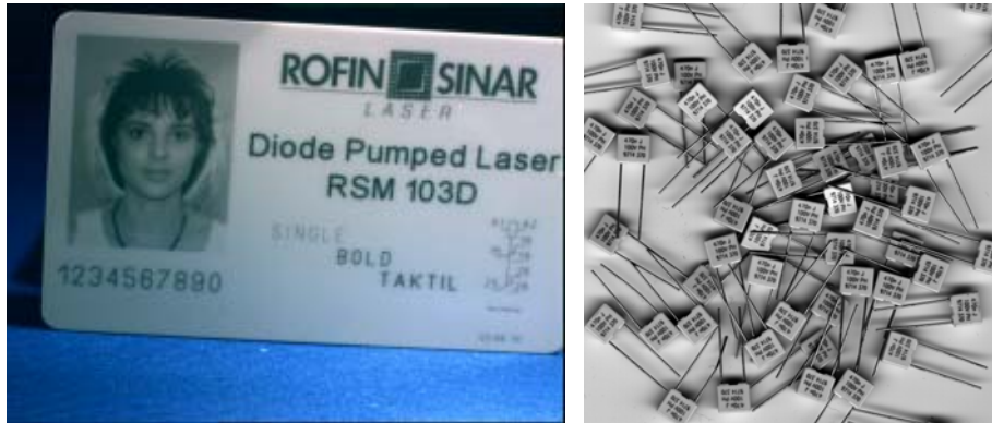
Figure 2.30: Left, PS carbonisation [Nd:YVO 4 , pulse width \approx 8 ns, 1064 nm], source: Rofin Sinar. Right, high speed component marking, PBT + glass fibre, [Nd:YAG laser].
