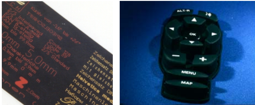
Figure 2.26: Left, ablation of three-layer foil: black top-layer, yellow middle layer and base layer red, [Q-switched Nd:YAG]. Right, day and night technique, [Q-switched Nd:YAG].
