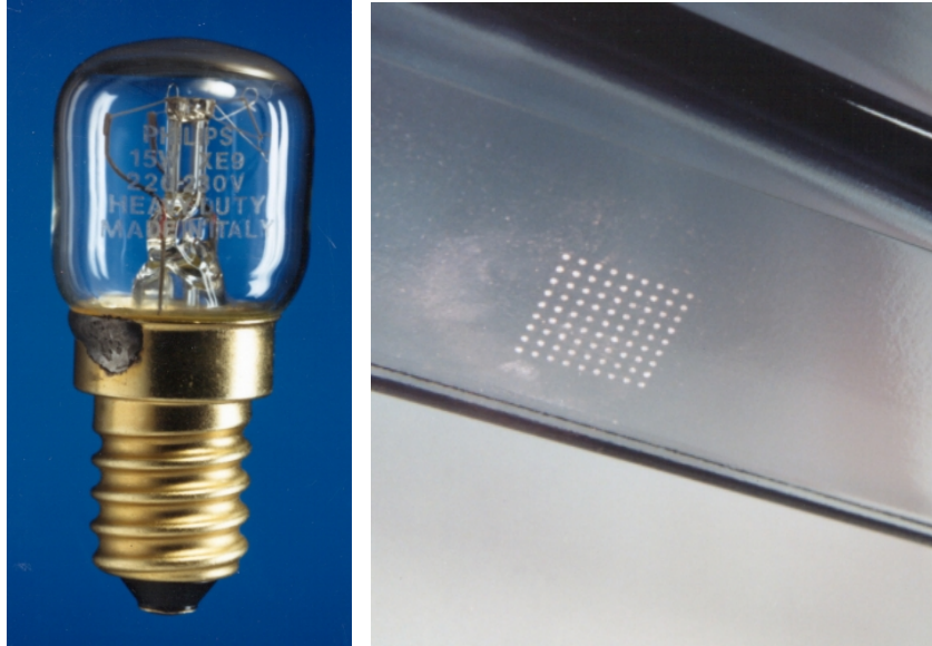
Figure 2.12: Left, ablative mark laser of incandescent lamp. Right, ablative mark for laser TV tube marking, both done by [TEA CO 2 ].
