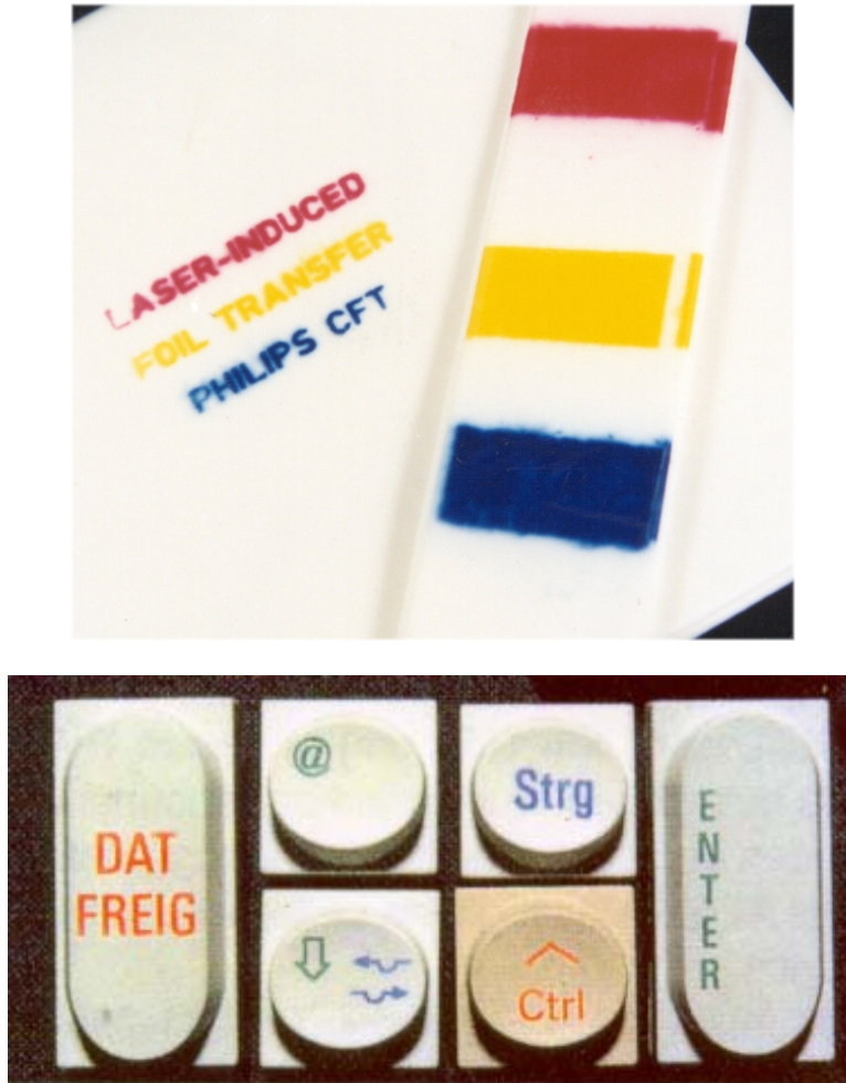
Figure 2.28: Top, laser-induced dye transfer, diffusion from foil into polymers, [CO 2 , laser]. Bottom, LIFT, multi colour marking by laser-induced foil transfer, source: Siemens [CO 2 , laser].
