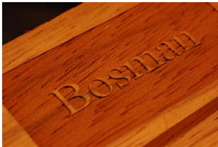
Figure 2.52: Sample of wood engraving [ 3^{\text{rd}} Nd:YAG, 355 nm].
