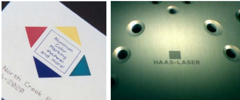
Figure 2.11: Left, anodised aluminium re-colouring, source: Synrad [ \text{CO}_2 laser]. Right, colour-forming in anodised aluminium, source: Philips DAP LTM(ATC) [Q-switched Nd:Vanadate].
