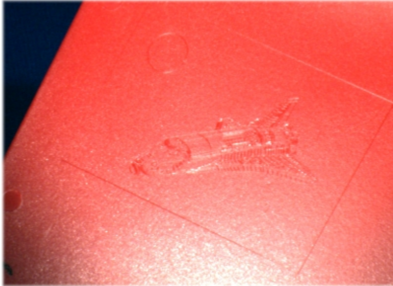
Figure 2.27: CO 2 laser mark in ABS.
