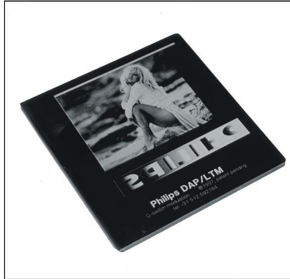
Figure 4.15: Written by inversion modulation with a second harmonic Nd:YAG on ABS, source: PHILIPS DAP-LTM, Martijn de Keijzer.
