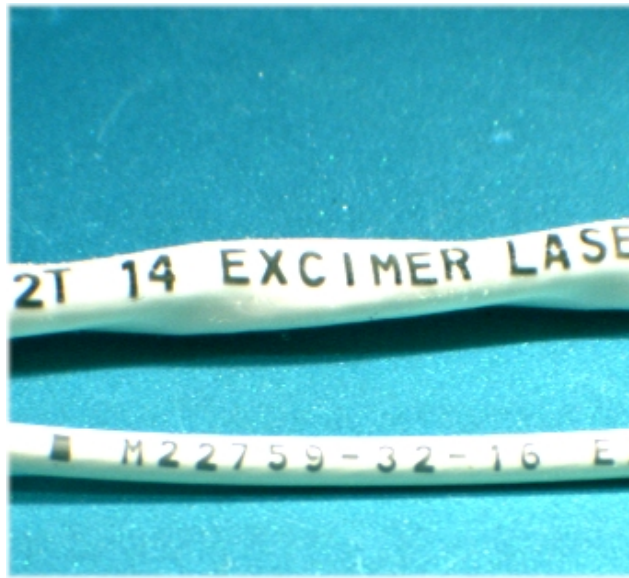
Figure 2.29: \text{TiO}_2 reduction marking of polymers, [Excimer 308 nm].
