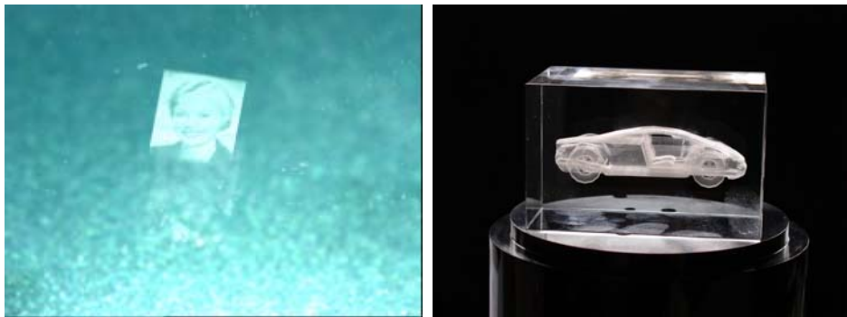
Figure 2.16: Left, in-glass marking set 2 mm below the glass surface, glass plate thickness 6mm, f\varnothing 160 mm, P \sim 0.5 W, Q 10 kHz, 10 pulses at one spot, Picture dimensions 4*3 mm, [3 rd harmonic Nd:YVO 4 ]. Right, 3D picture in glass, cube dimension 40x40x80 mm [3 rd harmonic Nd:YAG].
