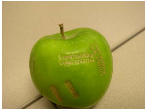
Figure 2.47: Marking of apples by skin ablation [ 3^{\text{rd}} Nd:YAG laser, 355 nm].
