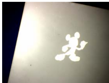
Figure 2.22: Al_2O_3 melting, photo taking in reflection, melted surface reflects the light to the camera. The area around the figure scatters the light [10 W CO_2 laser].
