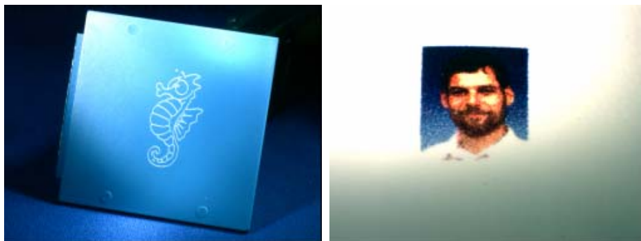
Figure 2.36: Left, polymer transfer [ \text{CO}_2 laser]. Right, 3 colour ablation transfer by [ 2^{\text{nd}} Q-switched Nd:YAG laser, 532 nm].
