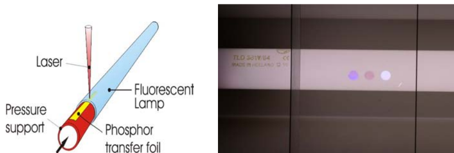
Figure 2.24: Blue and red phosphor transfer inside a fluorescent lamp. Left, principle setup. Right, fluorescent lamp with transferred blue and red circles. The third and most right circle is only cleaned using laser ablation.
