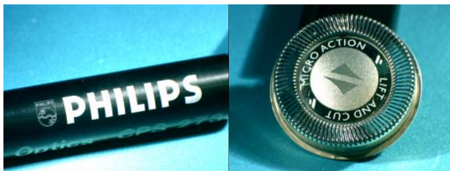
Figure 2.5: Left, anodised aluminium ablation [2 nd Q-switched Nd:YAG, 532 nm]. Right, grey logo in the middle is applied by re-growth of previously ablated anodised layer on Aluminium [Q-switched Nd:YVO 4 ].
