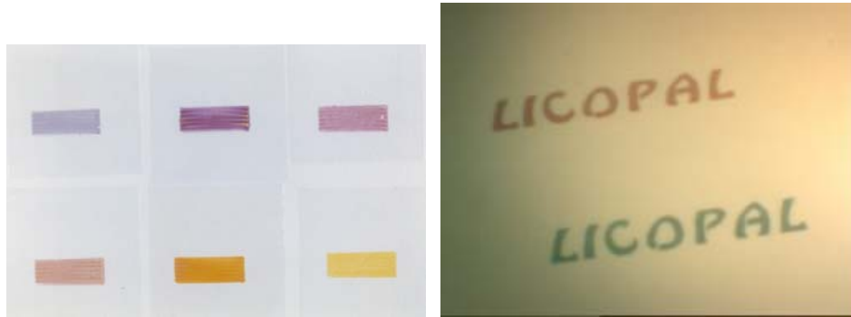
Figure 2.35: Left, thermal colour-formers in lacquer [ \text{CO}_2 laser]. Right, UV colour-former,[excimer, 351 nm].
