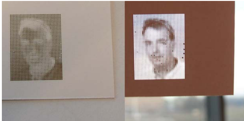
Figure 2.44: Picture with low resolution but large grey scale range cut in paper width of picture 20 mm. With backlight (right) and without backlight illumination (left). [3 rd harmonic Q-switched YAG].
