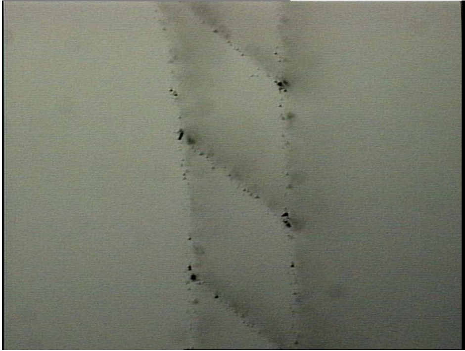
Figure 3.11: Locally degraded PC (horizontal distance between the two vertical lines 0.5 mm)
