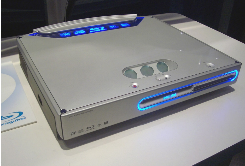
Figure 2.17: Blu-Ray recorder Philips, top backside full in glass marking with blue led illumination [3 rd harmonic Nd:YAG].
