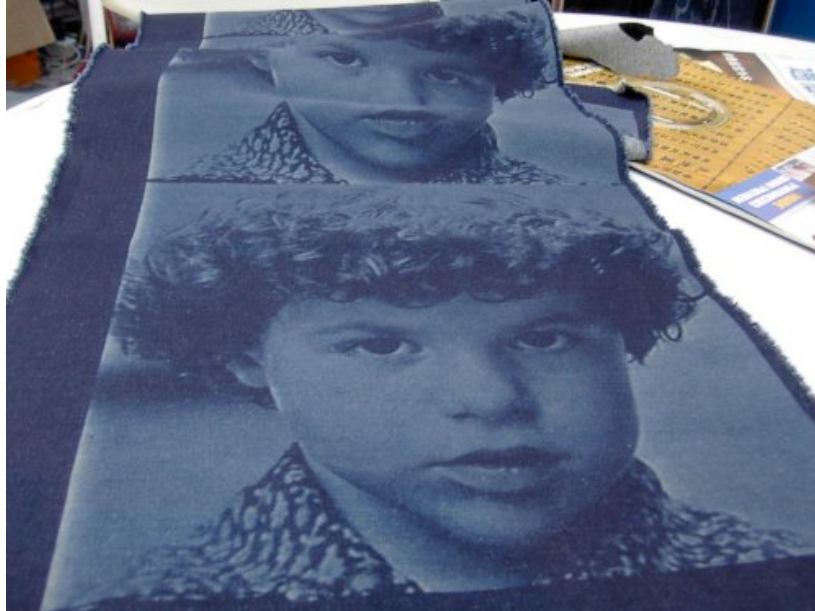
Figure 2.54: Bleached jeans, source: DS4 [sealed CO 2 laser, 10.6 μm].
