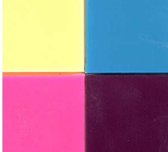
Figure 6.15: Top left, plate 4, ABS + cromophtal yellow HRP. Top right, plate 10, ABS + cromophtal blue 4GNP. Down left, plate 7, ABS + cinquasia mag. RT-235 D. Down right, plate 19, ABS + cromophtal yellow HRP+ cinquasia yag. RT-235 D + cromophtal blue 4GNP
