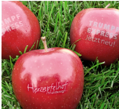
Figure 2.50: Bleaching of apples, source: Trumpf [3 rd Q-switched Nd:YAG laser, (355 nm)].
